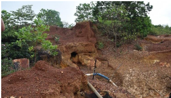
Above: Burrowing into the side of pit walls dramatically raises the likelihood of cave-in.
