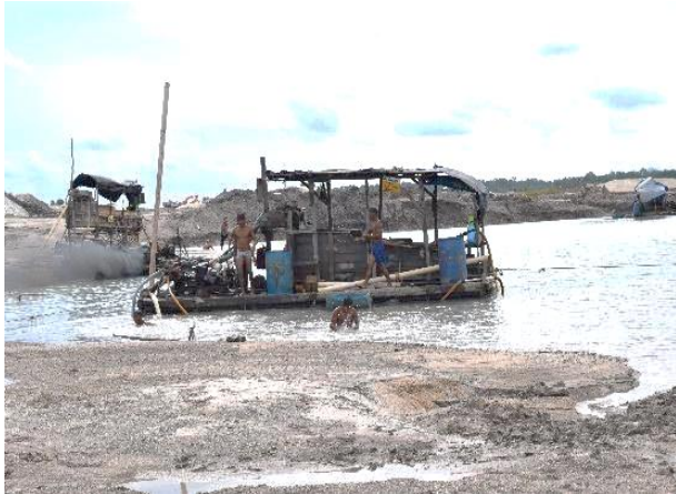
Above: Pontoon (raft used for mining) crew use the PVC tube with a steel spearhead to pierce the bottom of the pit. The ore is then suctioned up and concentrated using the sluice onboard and onshore.
