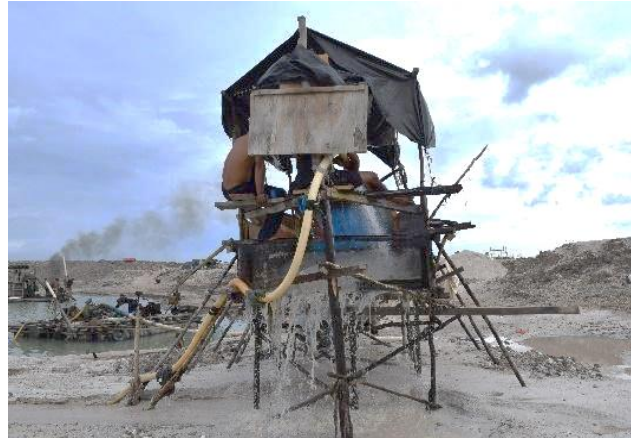
This sluice processes the cassiterite ore from the pontoon raft.
